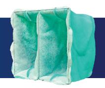
**Cube Filters** are manufactured with two layers of synthetic media. The upstream layer consists of larger fibers with a more open structure for greater depth loading, excellent dust holding capacity that will lead to a longer life. The final layer consists of fine bi-component fiber for capturing fine particles. The final layer is thermally bonded and contains no chemical binders.
